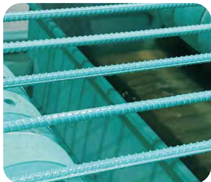
Rebar in Epoxy surface 环氧表面钢筋
